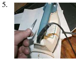
Cover the knife back up with paper and put the iron on top. Let it cook for 2-1/2 to 3 minutes. When you uncover the knife, the Press-N-Peel should have turned from a pastel blue color to midnight blue ... that seems to indicate that the resin has been melted onto the metal.
