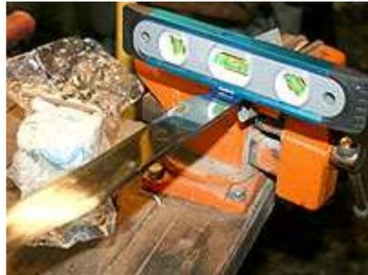
Now we're getting down to brass tacks. Use the vice and the level to get the etch area good and flat. I've found that if I am a little off, and my pool of etchant is deeper on one side – that side will also etch deeper.
