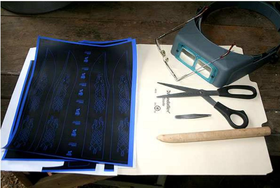
Magnifying glasses are good. Scissors are used to cut out the image you are going to apply. Tweezers are nice to handle the Press-N-Peel without getting it grubby. I've taken a piece of softwood dowel and ground one end to a slightly rounded shallow angle – I use this as a burnishing tool.
