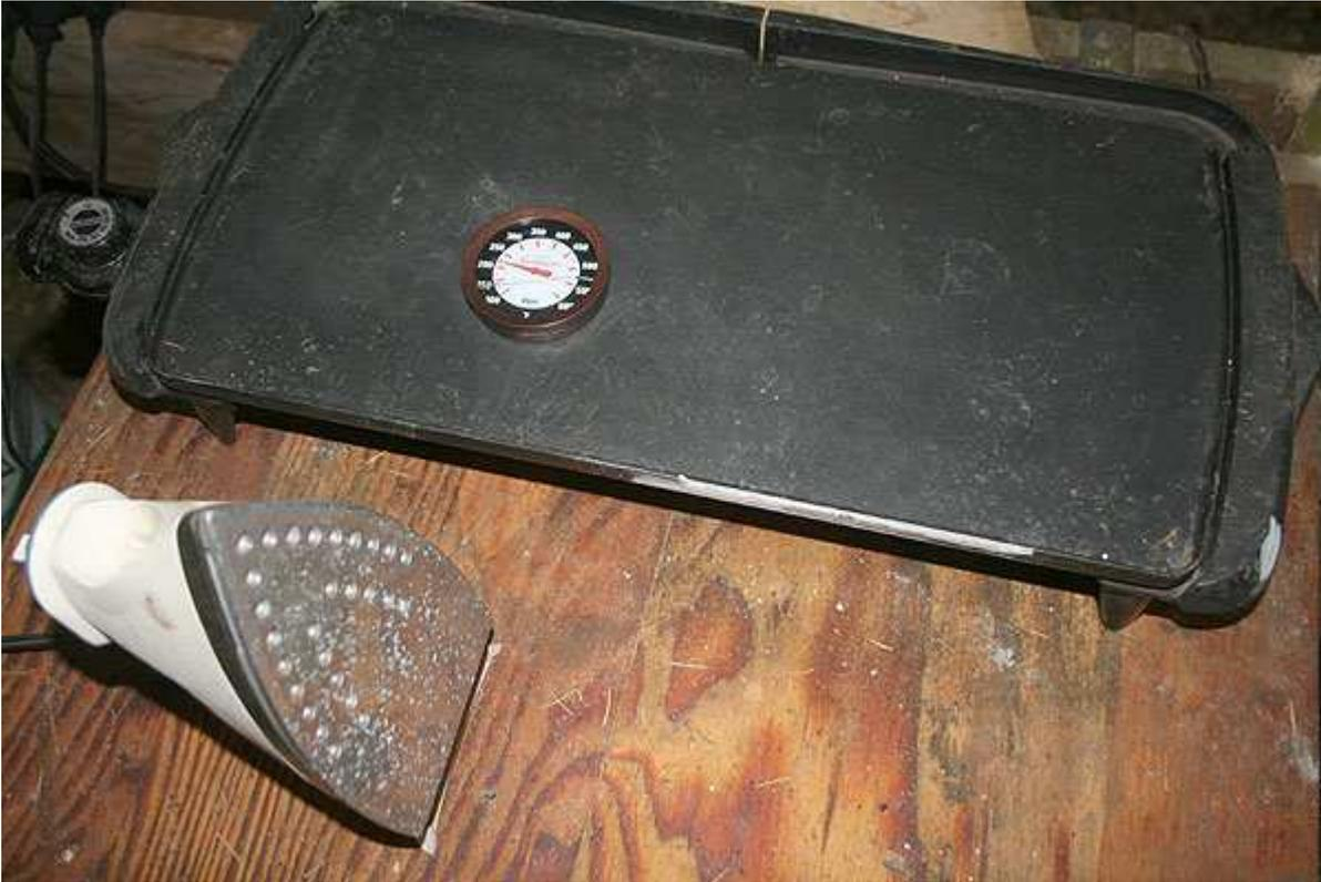
Yes – my setup is pretty funky! I set the griddle so that it is a little over 200°F – the oven thermometer shown here reads about 210°F. The iron is set somewhat higher – this old iron is set between wool and cotton – and the oven thermometer reads about 320°F if you let it sit on the iron.
