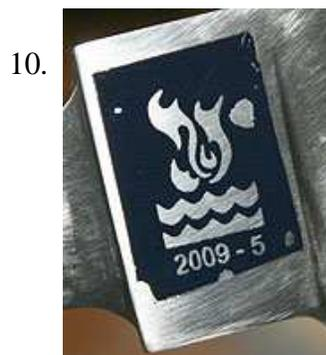
OK – after cleaning the blade and trying a second time – this is a mask that I can fix. All the voids are away from the text and graphics.
