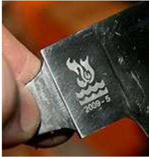
It is tricky to dump the acid out of the dam without getting it on other parts of the blade – but in any case, do this near a hose or other water supply which you can use to totally flush off all the acid. I believe that you could use baking soda to neutralize the acid – but I've never needed to bother with that.
