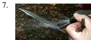
Next, spray the knife to cool it down – in this photo the blade was still too hot for me to hold barehanded so I've got it by a pair of pliers on the tang. The resin needs to be cold before you remove the plastic layer or it will smear (trust me – I've tried all the variations).
