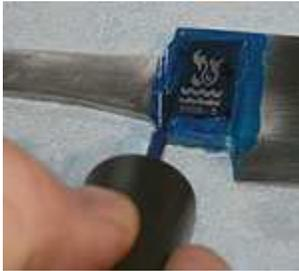
And after I've fixed the voids I use cheap fingernail polish to make a larger safe area for the etching. I've thinned the polish down with acetone to make it easier for me to apply.
